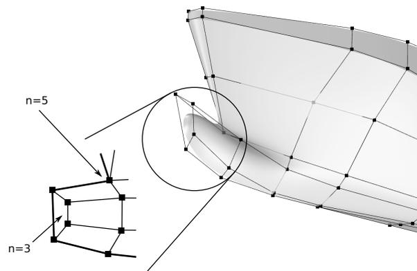
Figure 1: The illustrated control points define the shape of bulbous. If the bulbous bow is going to be optimized, it suffices to consider these points as parameters.
