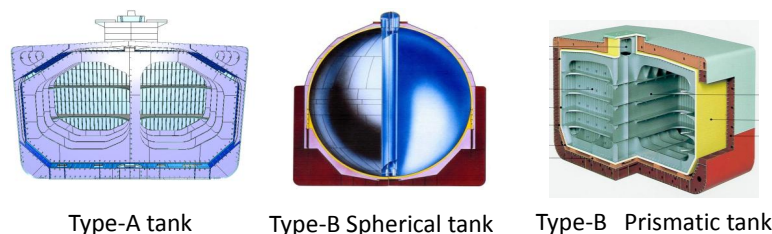
Figure 7: Cross sections of independent tank types A and B (with courtesy to DNV, Moss Maritime and IHI respectively)
