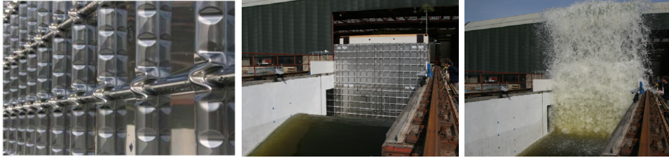
Figure 7: Quasi full scale impact experiments (Sloshel project)
