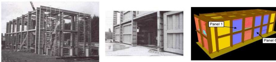
Figure 24: Spadeadam test site, offshore module and location of the panel during the test.
